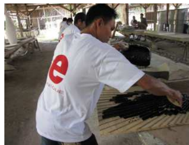
Local artist, Bayani applies the water based paint in the first step of the coating process.
